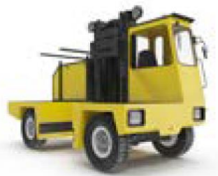
Fig. 5 Side loading lift truck
