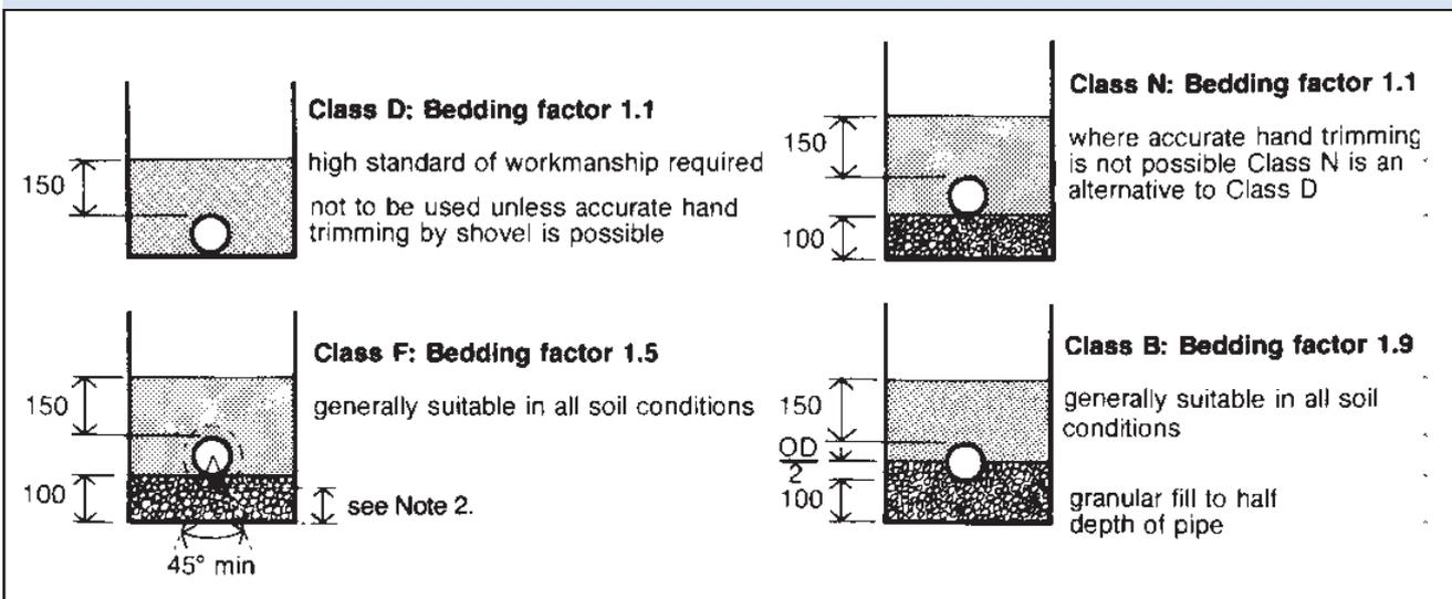
Diagram 9 Bedding for flexible pipes
