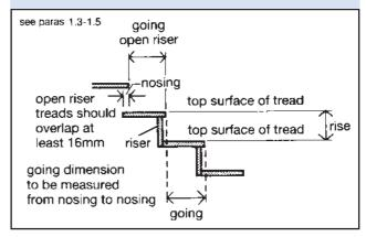
**1.5** The normal relationship between the dimensions of the rise and going is that twice the rise plus the going (2R + G) should be between 550mm and 700mm.
