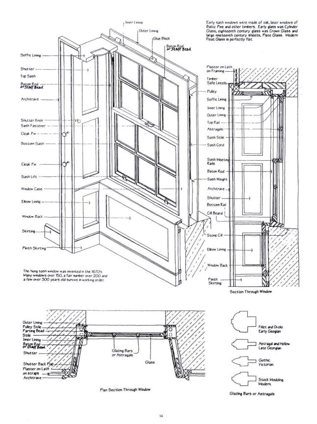
Figure: typical sash window and terminology
