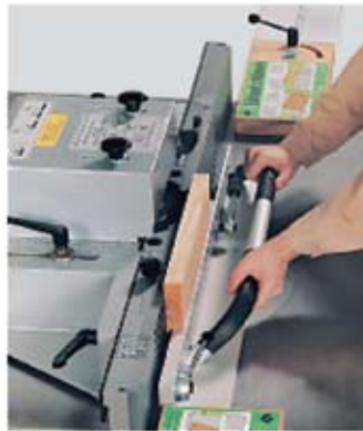
Use of jig for stopped work
