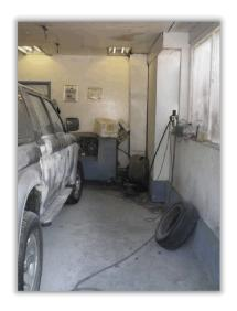
The use of this area for spraying vehicles, using highly flammable liquids, was stopped because there was unprotected electrical equipment in the vicinity of where spraying was taking place.
