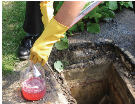
Oil contamination of a borehole
