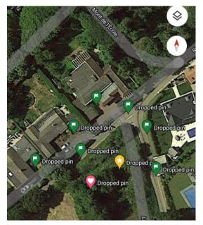
The red heart pin is the antenna location, the green flag pins are intermediate locations measured at during the peak search and the yellow star pin is the spot where the highest spot search reading was obtained and where the detailed survey was carried out During the 2022 survey, the emission levels were measured at 0.68% of ICNIRP, about 147 times smaller than the ICNIRP limits. This site is deemed to be safe and should not be a concern to the local residents or members of the public.
