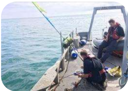
Fisheries Officers exchanging batteries and the SD card from a C-Pod after a successful 3 month deployment.
