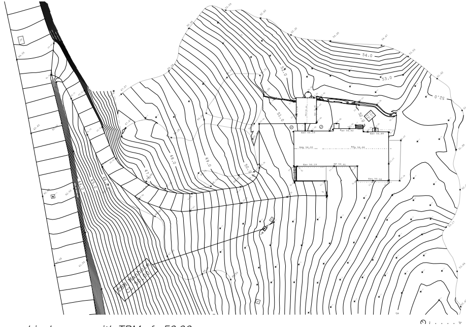
Topographical survey with TBM of +50.00
