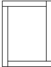
2. Staple the joins together using 3 – 5 staples per join on each side;
