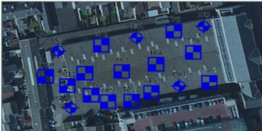
Figure 5 – Locations of Borehole Installations and Trial Pit Excavations [Geomarine]
