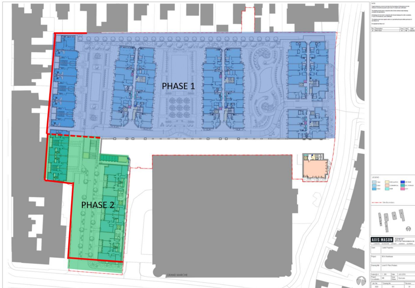
Figure 18 – Proposed Phasing of Remediation Works / E-Clay PRB Installation
