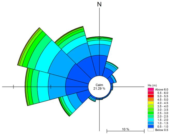
Figure F-4: Wave Rose at Jersey Wave Buoy (significant wave height, Hs)
