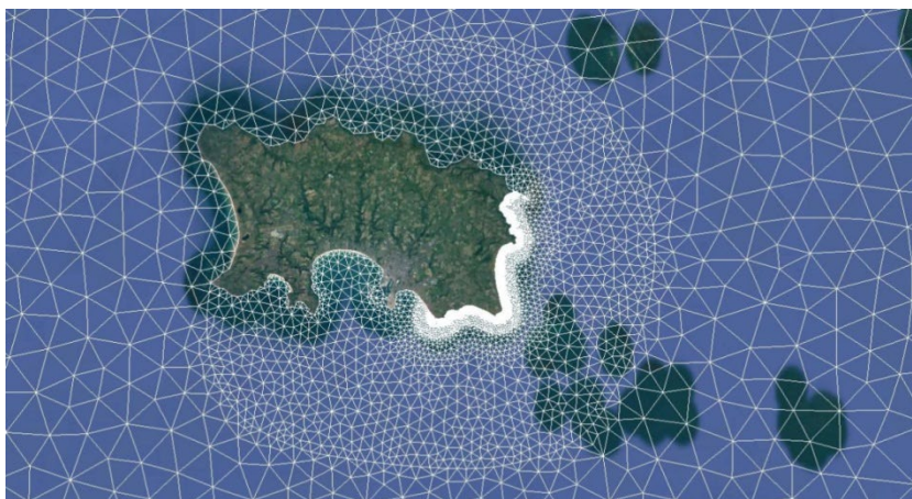
Figure G-16: View of Enhanced Nearshore Mesh Resolution along the East Coast (Model D)
