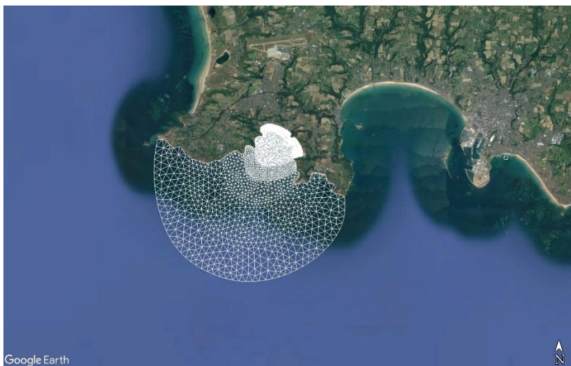
Figure G-13: Local Wave Model Mesh (Model C)
