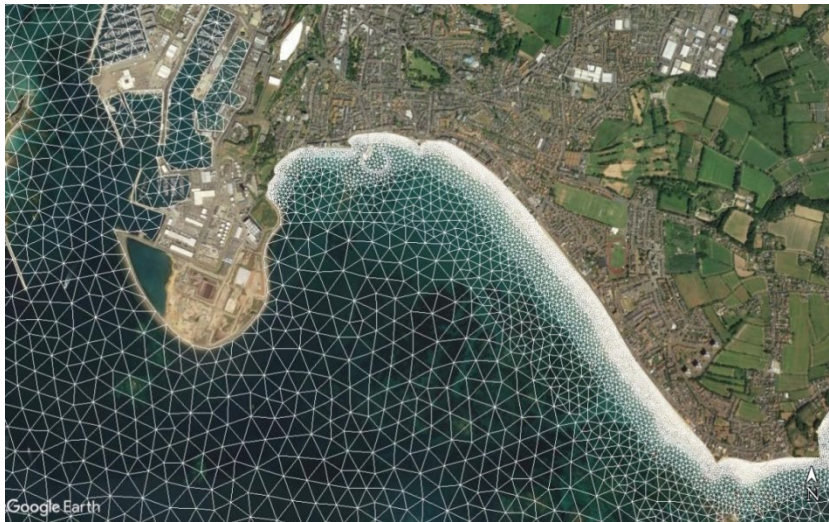
Figure G-12: View of Enhanced Nearshore Mesh Resolution (Model B)
