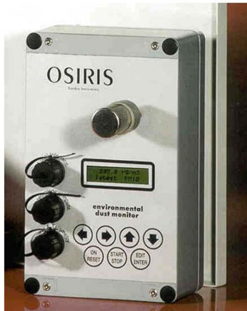
Photograph 1: Turnkey Osiris particle unit 9
