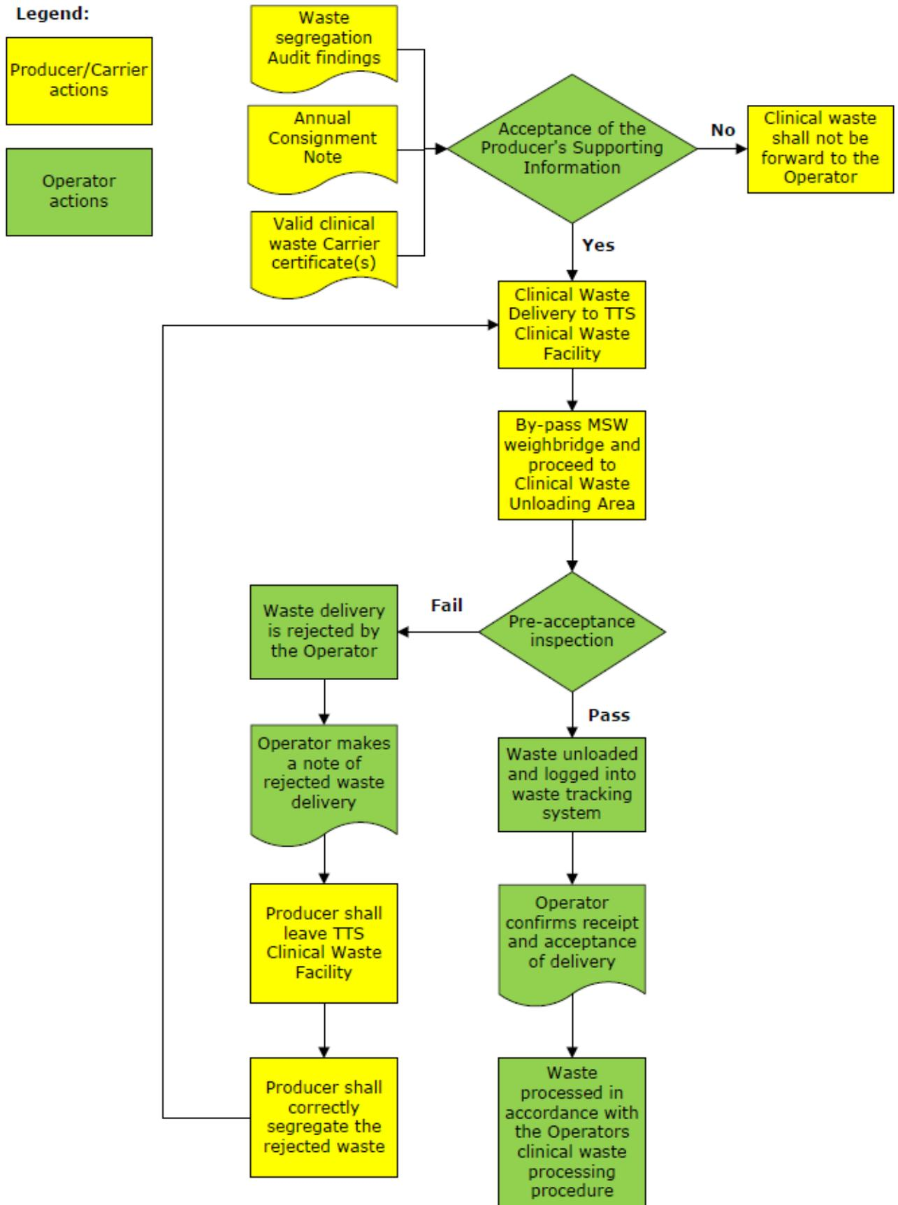
**Figure 1, Waste Acceptance Process Flow**
