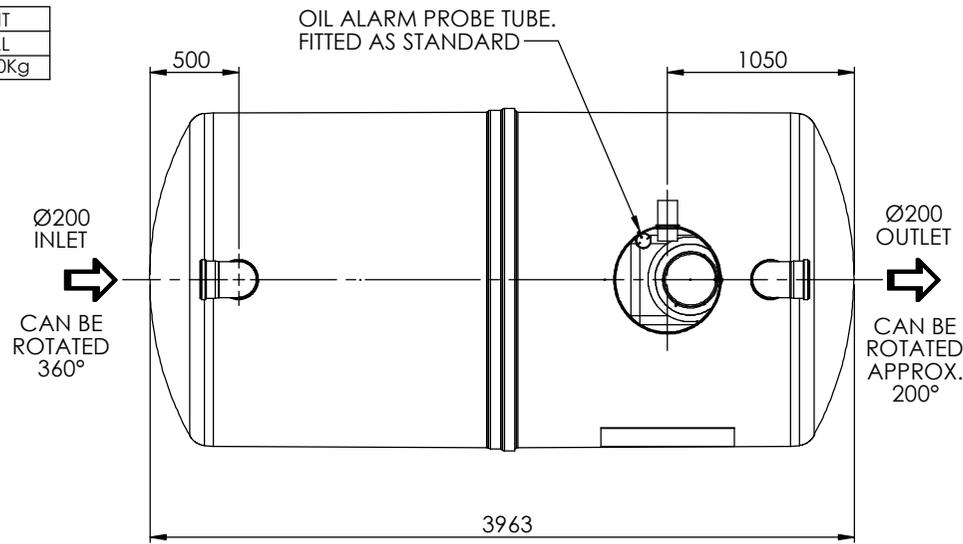
NOTE:- THE DESIGN OF THIS UNIT IS BASED ON AN NS20 FULL RETENTION UNIT
