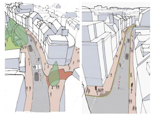
• mean the carriageway width is narrowed for the cycle lane, with westbound cyclists continuing to • be a mandatory cycle lane denoted by a solid white line, prohibiting motorists from entering it and • mean the unloading bay and parking next to Morier House will be removed. The unloading bay to
