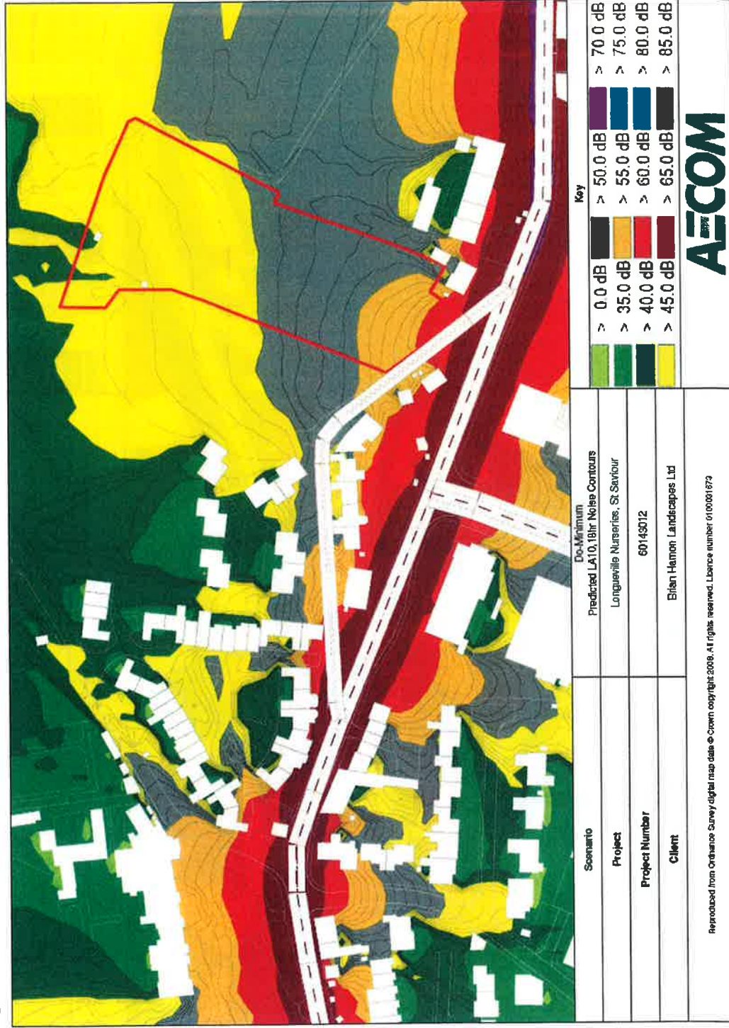
Figure D.3: Do-Minimum L_{A10,18h} Noise Contour Plot
