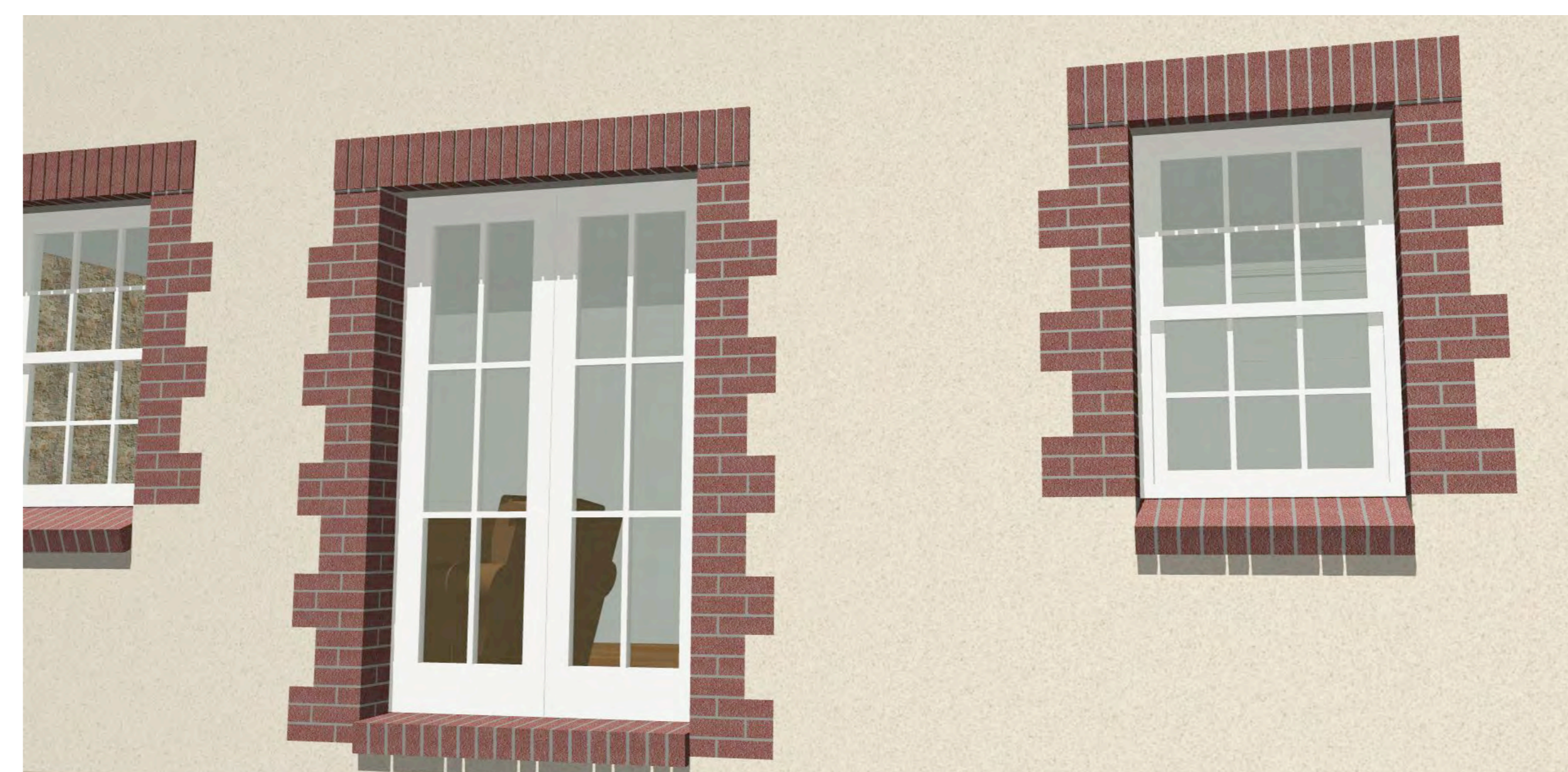
TYPICAL FRENCH DOORS & WINDOWS TO GARDEN WITH BRICK QUIONS AND LINTOL IN PAINTED RENDER FINISHED WALLS. SEE DWG 1871/P/02. TYPICAL WINDOWS SEE 1871/P/01
