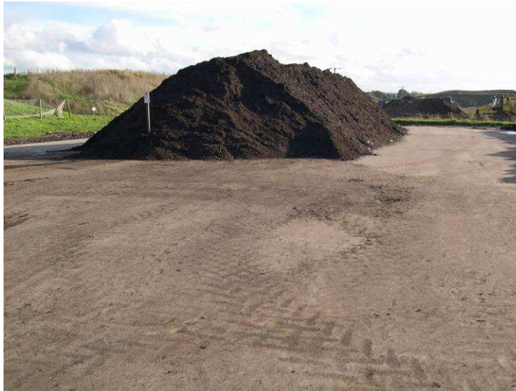
Figure 8 Solid digestate maturing in windrows on a secure concrete storage area
