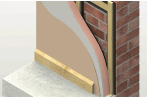
Diagram showing installation of internal wall thermal insulation
