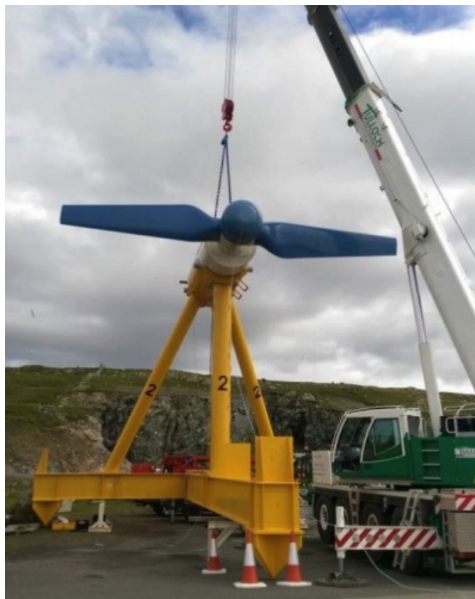
Figure 5, Nova's M100 prior to deployment at Bluemull Sound, Shetland
