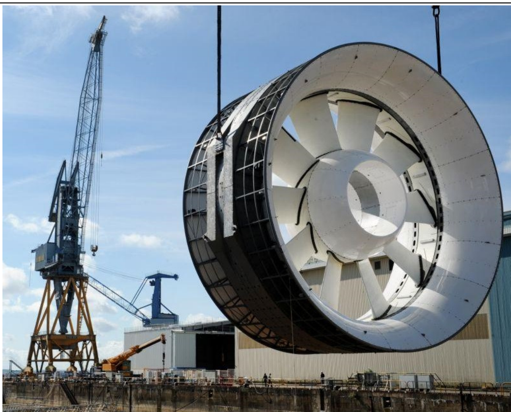
Figure 7, OpenHydro's turbine prior to deployment in Brittany, France
