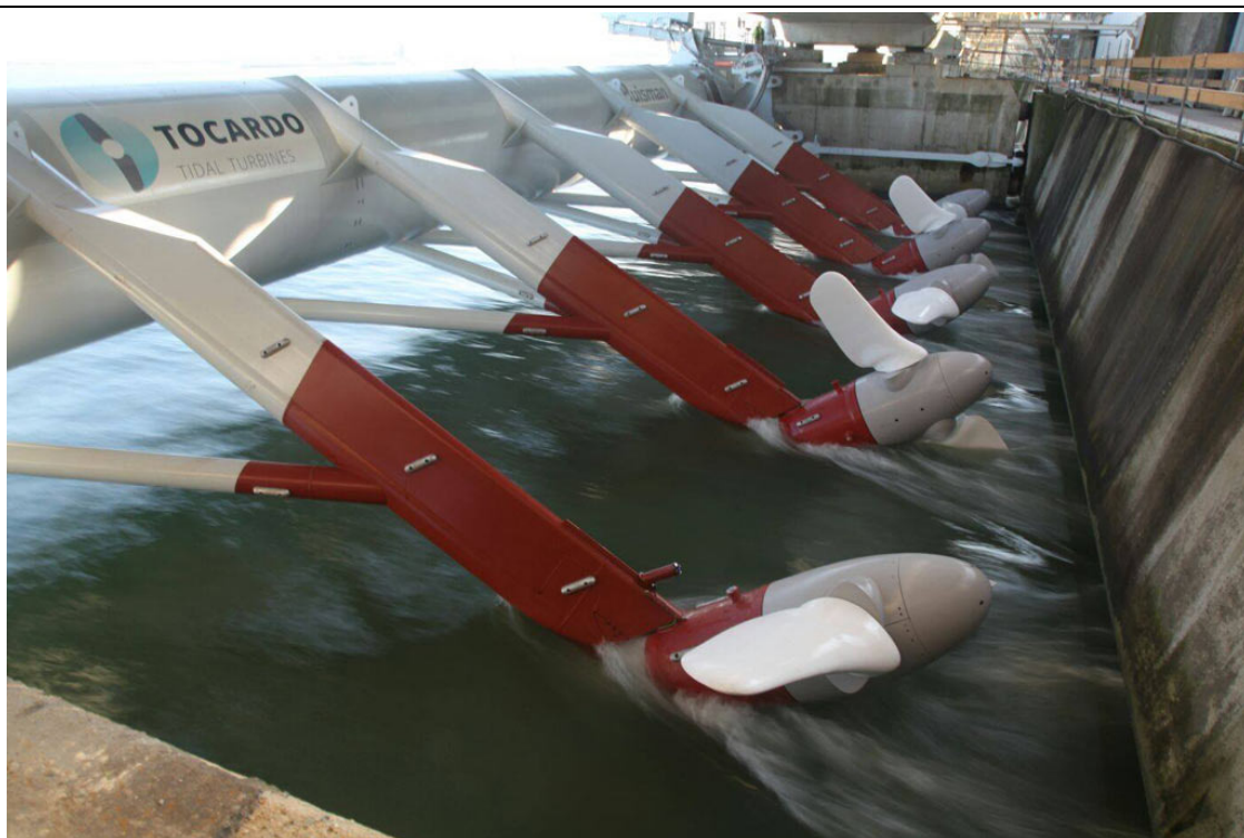
Figure 8, Five 250kW Tocardo T2s installed in the Oosterschelde, Netherlands
