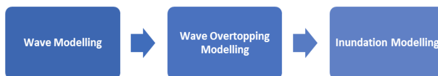
Figure 2-2: Modelling procedure for coastal flooding assessments
