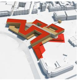
Further future expansion could be accommodated through vertical extension of the roof zone. This will require prvisions to be made in the building structure and vertical communication strategy.
