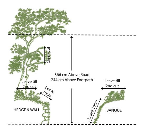
Metric Measurements Above Road clearance height 366 cm Above Footpath clearance height 244 cm
