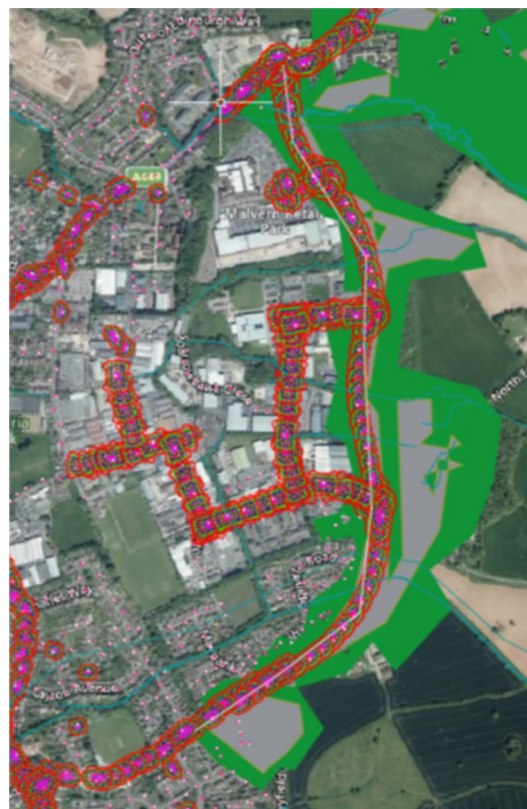
Figure 15. An illustration of some of the mapping, monitoring and assessment of existing lighting levels. Trunk road lighting interacts here with a broadleaved woodland component of the local ecological network. Image © Crown copyright and database rights 2023 Ordnance Survey 100024230, © Getmapping Plc and Bluesky International Ltd 2023.
