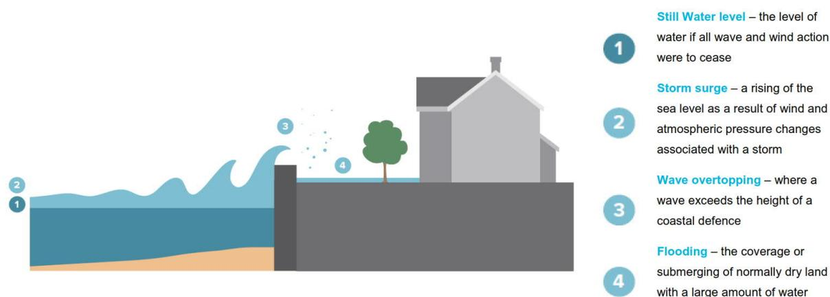
Figure 3-1 Summary of coastal flooding mechanisms<sup>7</sup>
