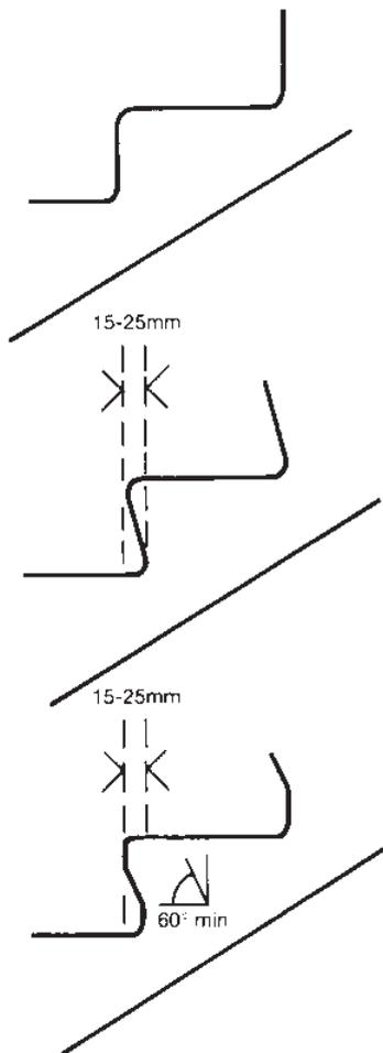
B. EXAMPLES OF SUITABLE TREAD NOSING PROFILES
