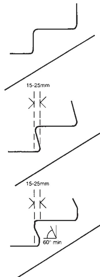
B. EXAMPLES OF SUITABLE TREAD NOSING PROFILES
