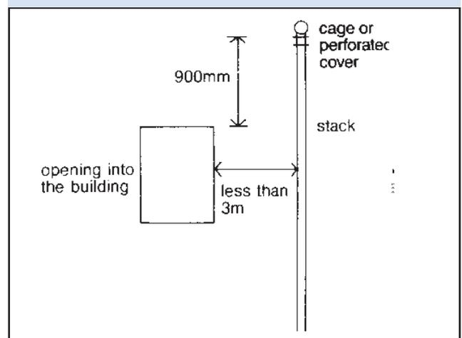
**1.26 Stub stacks** – An unventilated stub stack may be used if it connects above ground into a ventilated discharge stack or into a drain not subject to surcharging and no branch into the sub stack is more than 2m above the invert of the connection or drain and no branch serving a closet is more than 1.5m from the crown of the
