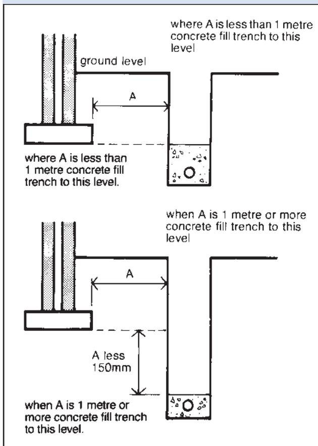
(b) where the trench is further than 1m from the building, the trench is filled with concrete to a level below the lowest level for the building equal to the distance from the building, less 150mm.
