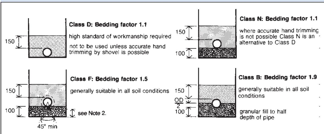
Diagram 9 Bedding for flexible pipes
