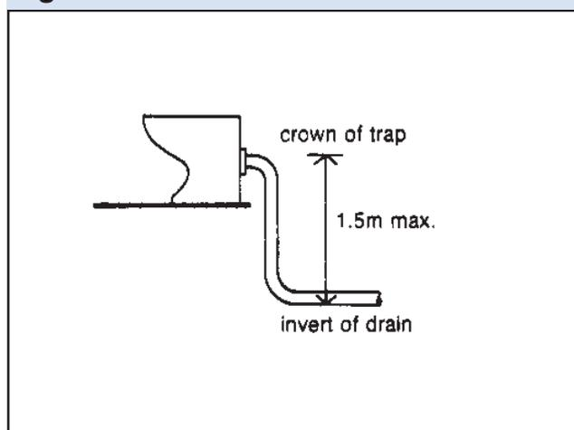
**1.6** If the appliances are on the ground floor the pipe(s) may discharge to a stub stack or discharge stack, directly to a drain, or (if the pipe carries only waste water) to a gully. (See paragraphs 1.9 and 1.2).
