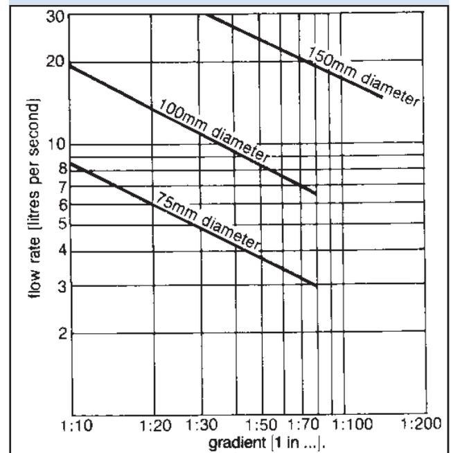
**2.11** A drain carrying only waste water should have a diameter of at least 75mm and a drain carrying soil water or waste water containing trade effluent a diameter of at least 100mm.
