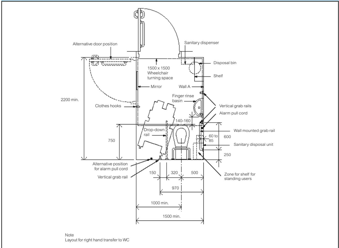
j. where the horizontal support rail on the wall adjacent to the WC is set with the minimum spacing from the wall, an additional drop-down rail is provided on the wall side at a distance of 320mm from the centre line of the WC;
