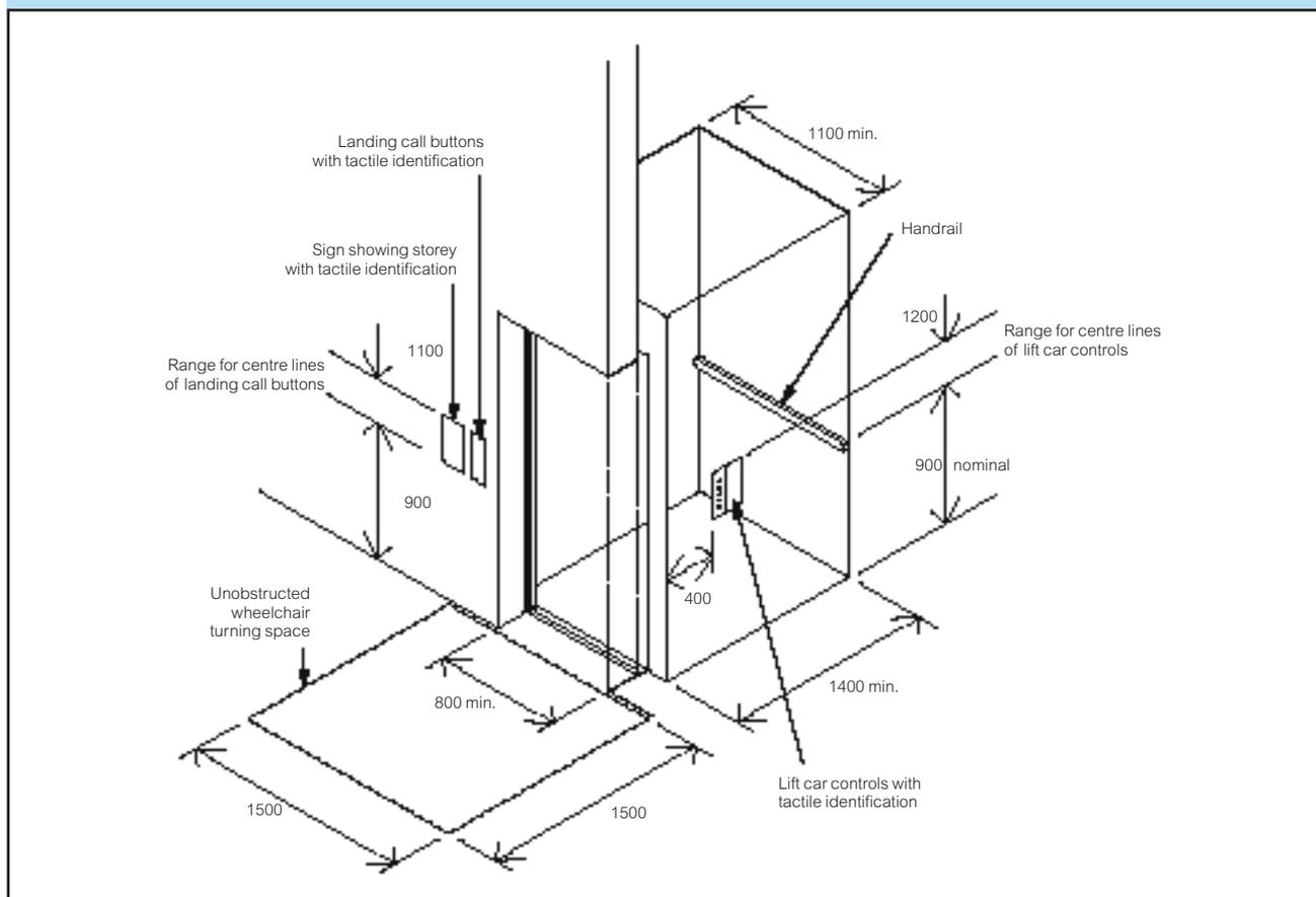
c. the minimum dimensions of the lift cars are 1100mm wide and 1400mm deep (see Diagram 11);
