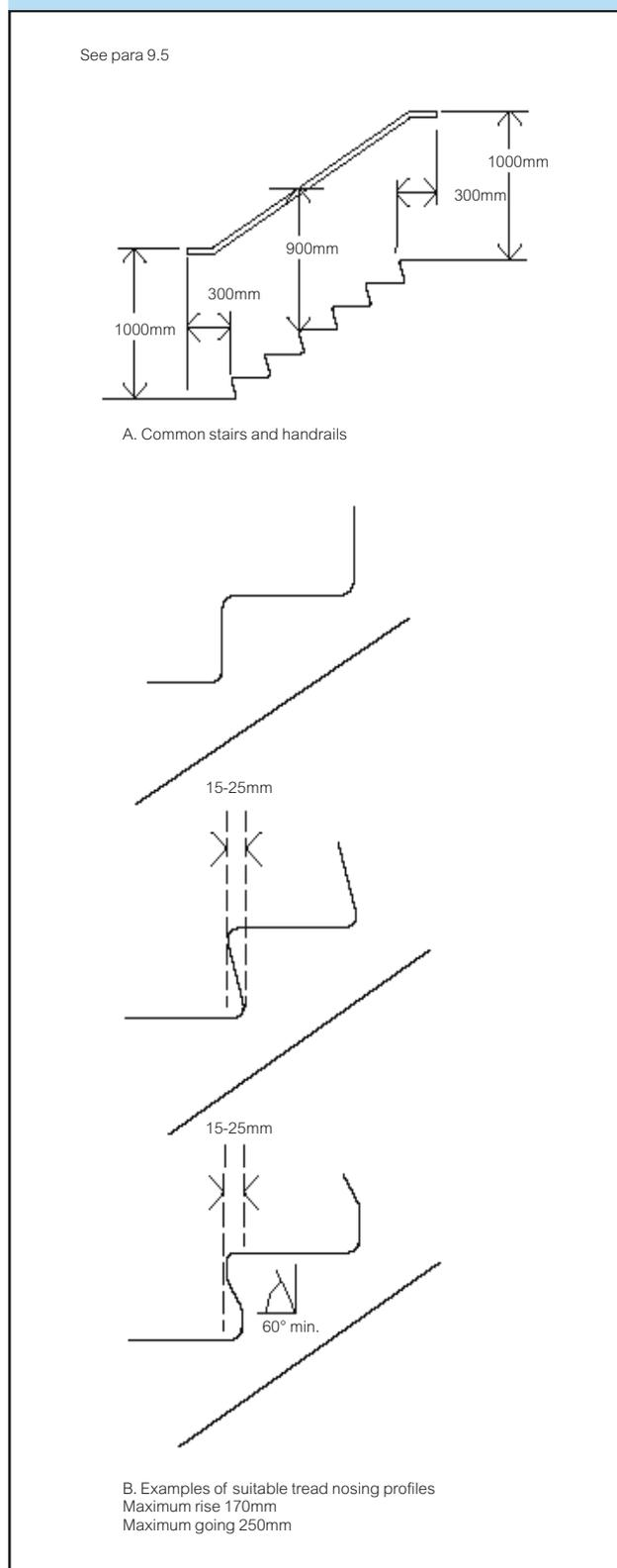
**9.6** Requirement 8.1 will be satisfied if a building containing flats, in which a passenger lift is to be installed, is provided with a stair that meets the guidance in the TGD Part 7 and all step nosings are distinguishable through contrasting brightness.
