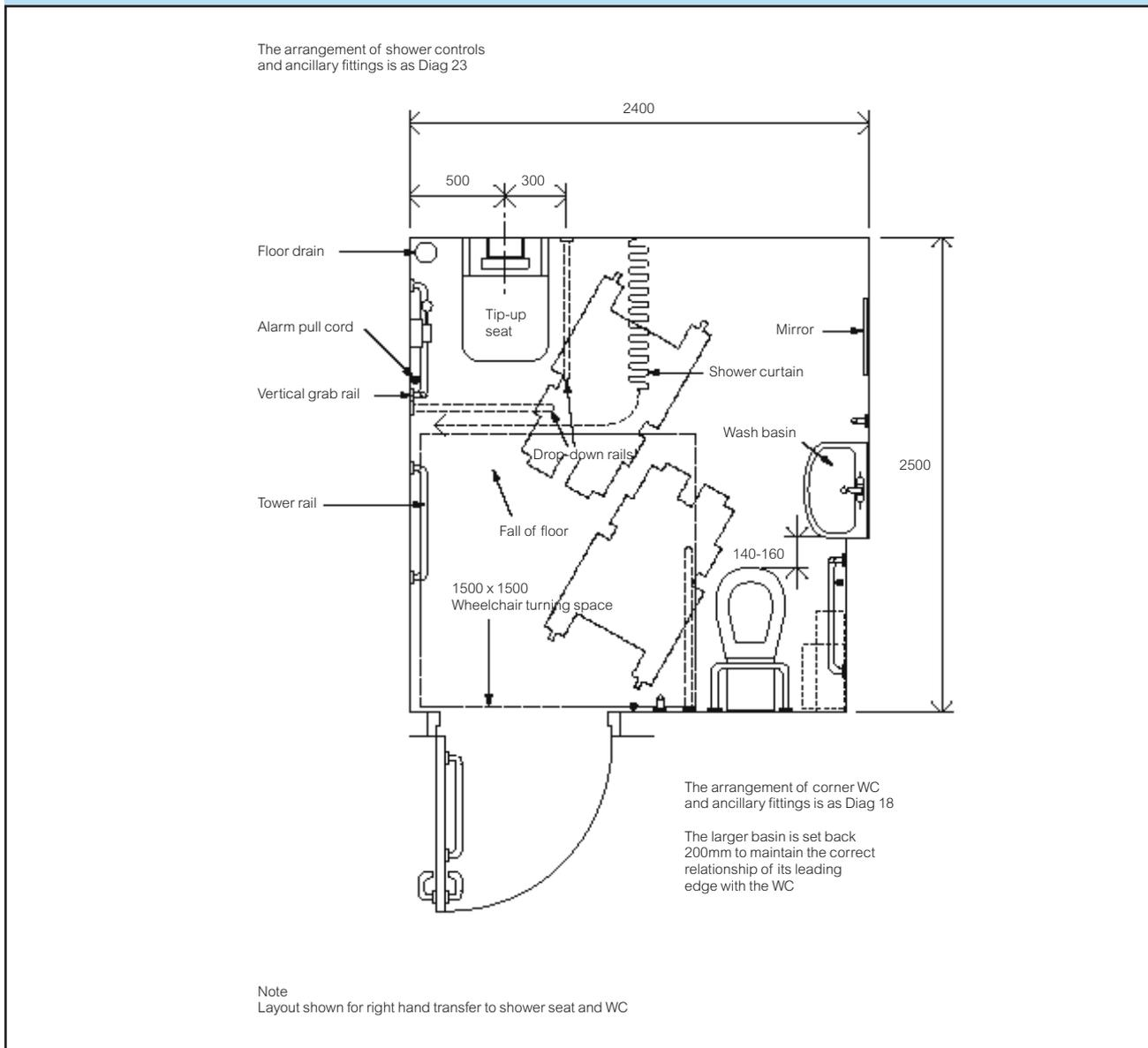
Diagram 25 An example of a bathroom incorporating a corner WC
