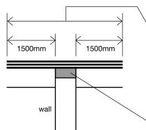
Roof covering over this distance to be designated AA, AB or AC on deck of material of limited combustibility. Roof covering and deck could be composite structure, eg profiled steel cladding.
