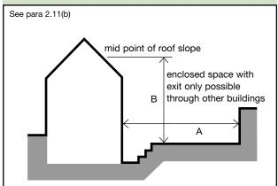
Depth of back garden A should exceed the height B of the house above ground level for it to be acceptable for an escape route from the ground or basement storey to open into the garden.
