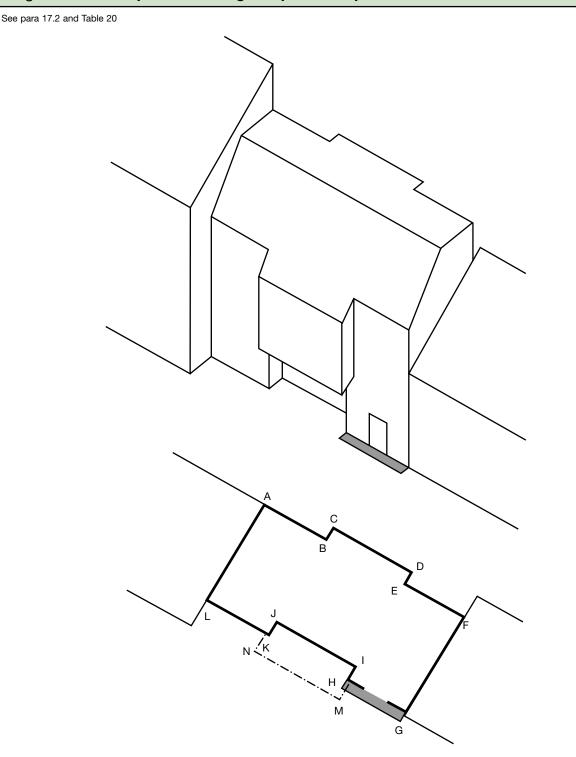
Plan of building AFGL where AL and FG are walls in common with other buildings.
