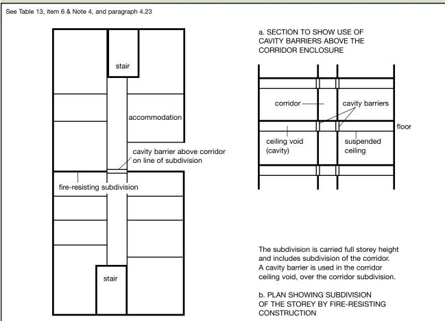
**10.5** As compartment walls should be carried up full storey height to a compartment floor or to the roof as appropriate, see paragraphs 9.22-9.25, it is not appropriate to complete a line of compartmentation by fitting cavity barriers above them. Therefore it is important to continue the compartment wall through the cavity to maintain the standard of fire resistance.
