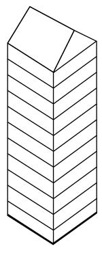
In a building over 30m in height all storeys should be separated by compartment floors. For advice on the special conditions in atrium buildings see B5588: Part 7.
