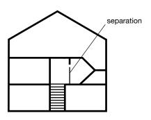
c. stair to new storey is in space converted and separated from first floor accommodation. New storey open to new stair. New stair separated from original stair at first floor level.
