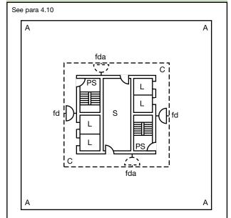
Note: The doors at both ends of the area marked 'S' should be self-closing FD20S fire doors unless the area is sub-divided such that any fire in that area will not be able to prejudice both sections of corridor at the same time. If that area is a lift lobby, doors should be provided as shown in Figure 8 in BS 5588: Part 11: 1997.
