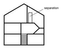
b. stair to new storey is in space converted and separated from first floor accommodation. New storey separated from stair at top level.
