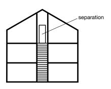
a. stair to new storey is within existing stairway. Separation of accommodation on new storey from stair is at top level.
