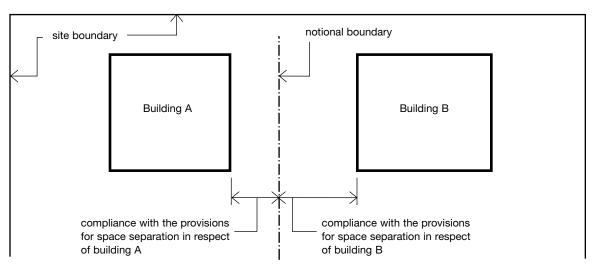
The notional boundary should be set in the area between the two buildings using the following rules:
