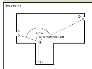
Angle ABD should be at least 45° plus 2.5° for each metre travelled in one direction from point C. CBA or CBD (whichever is less) should be no more than the maximum distance of travel given for alternative routes, and CB should be no more than the maximum distance for travel where there are no alternative routes.
