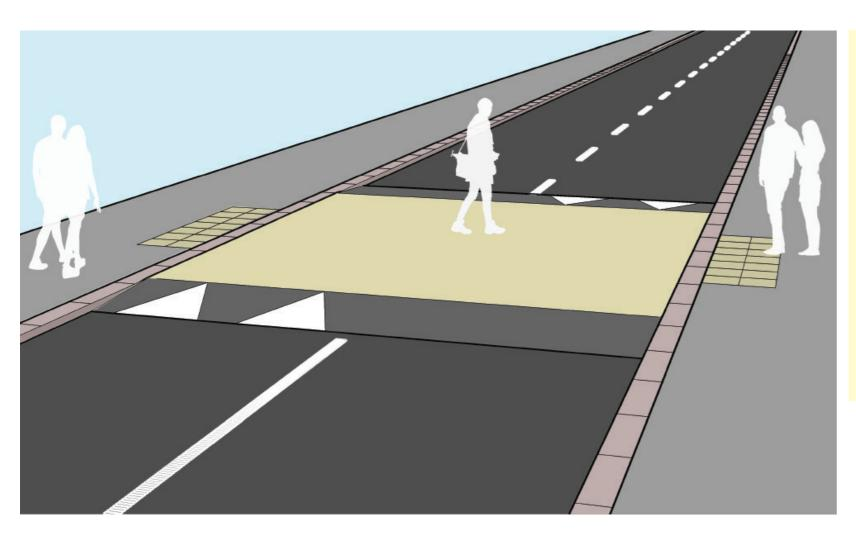
The five new crossing locations will each take the form of a raised table, with a 6m road length and ramps on each side. These are designed to slow traffic but without creating an unnecessarily abrupt deflection or noise effects and to accommodate the bus service. They also provide a level surface from pavement to pavement. Chevron markings on the ramps alert approaching drivers.
