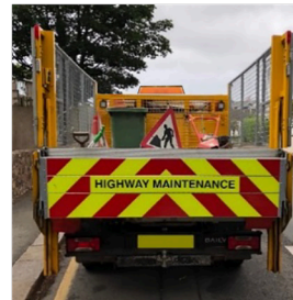
Example of works vehicles fitted with chevron markings and warning lights
