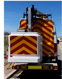
Example of works vehicles fitted with chevron markings and warning lights
