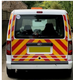
Example of works vehicles fitted with chevron markings and warning lights
