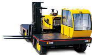
Fig. 5 Side loading lift truck
