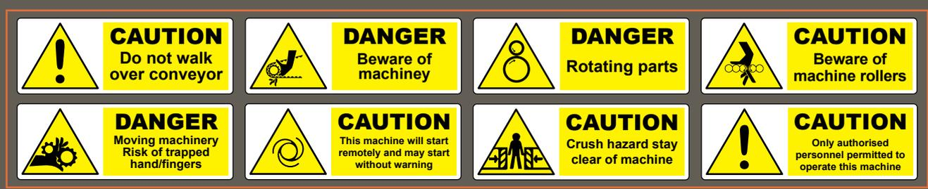
**32** All machinery should be marked with highly visible and indelible labels to provide warnings and raise awareness relating to the safe use of equipment. Pictograms are often used to represent particular hazards via symbols and pictures.
