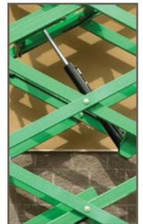
Machine parts that may cause crushing
