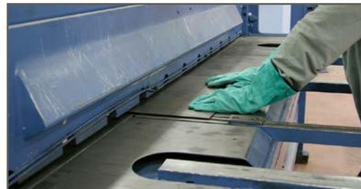
Machine parts that may cause shearing
