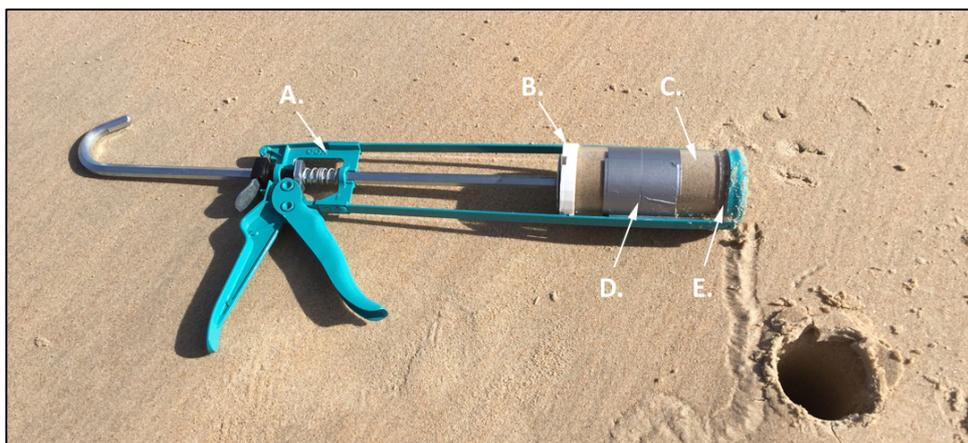
Figure 1. Coring frame (A.) with 3D printed endcap (B.) containing a 300-micron stainless steel mesh disc, and 2 stacked 5cm high Perspex cylinders (C.) secured at the mid-point (D.) with heavy duty Duct Tape. An additional 3cm Perspex buffer (E.) was permanently secured to the end of the coring frame.
