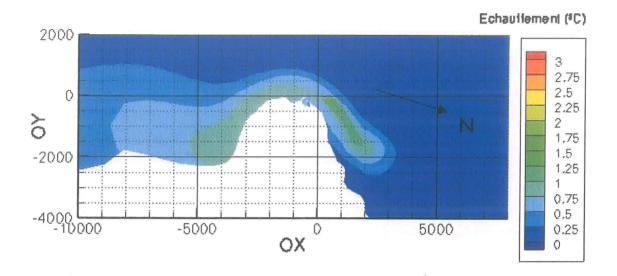
Modelling of the three units' maximal thermal plume off the cove shore of Sciotot by low tide
