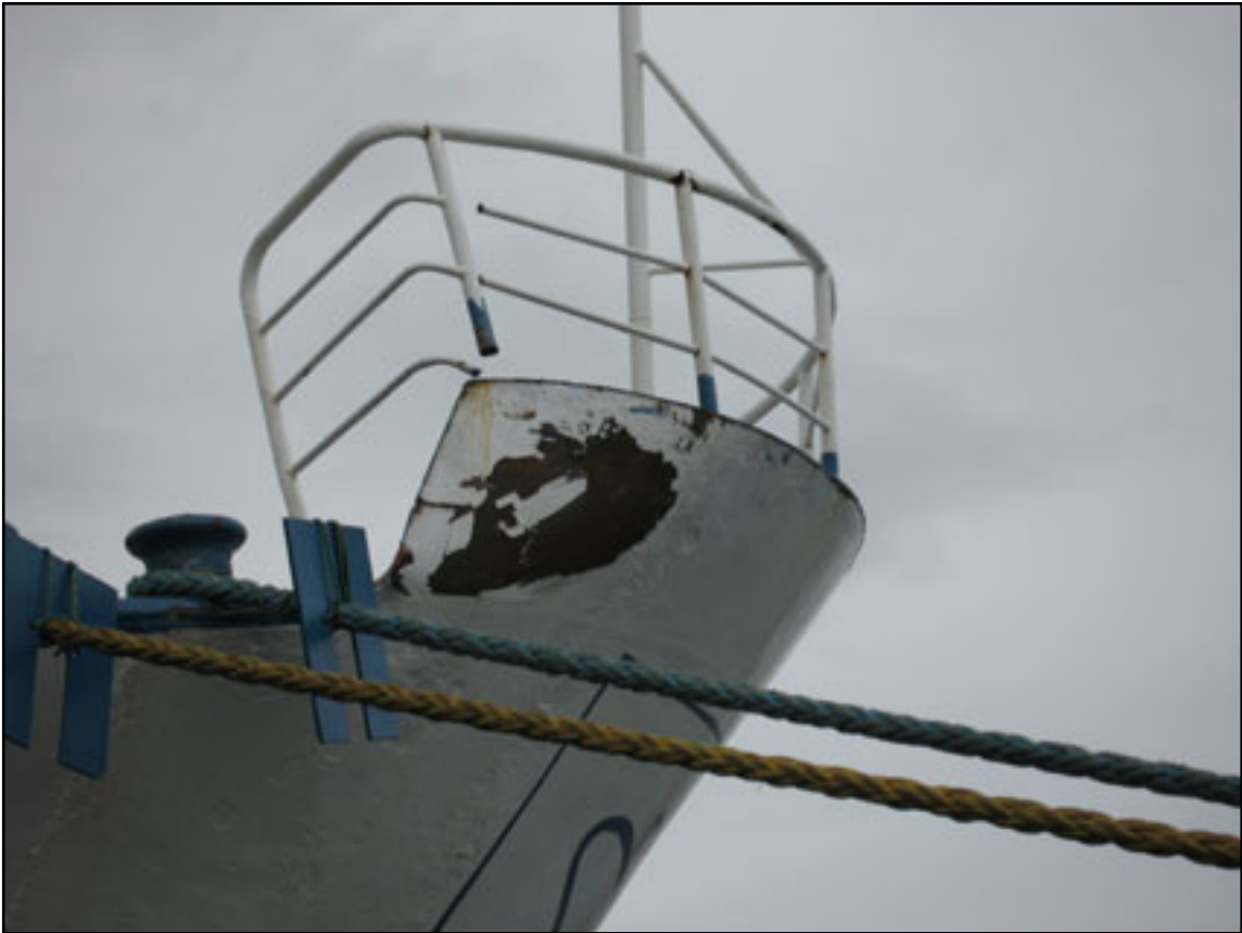
Damage to starboard bow of Logos II
