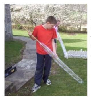
5. Stack the bottles one inside another with a garden cane supporting them through the middle. At one end reverse a bottle so it faces the opposite way from the rest and fit it inside. This will to make a long tube with the ends of the garden cane sticking out of the tops of the bottles at either end.
