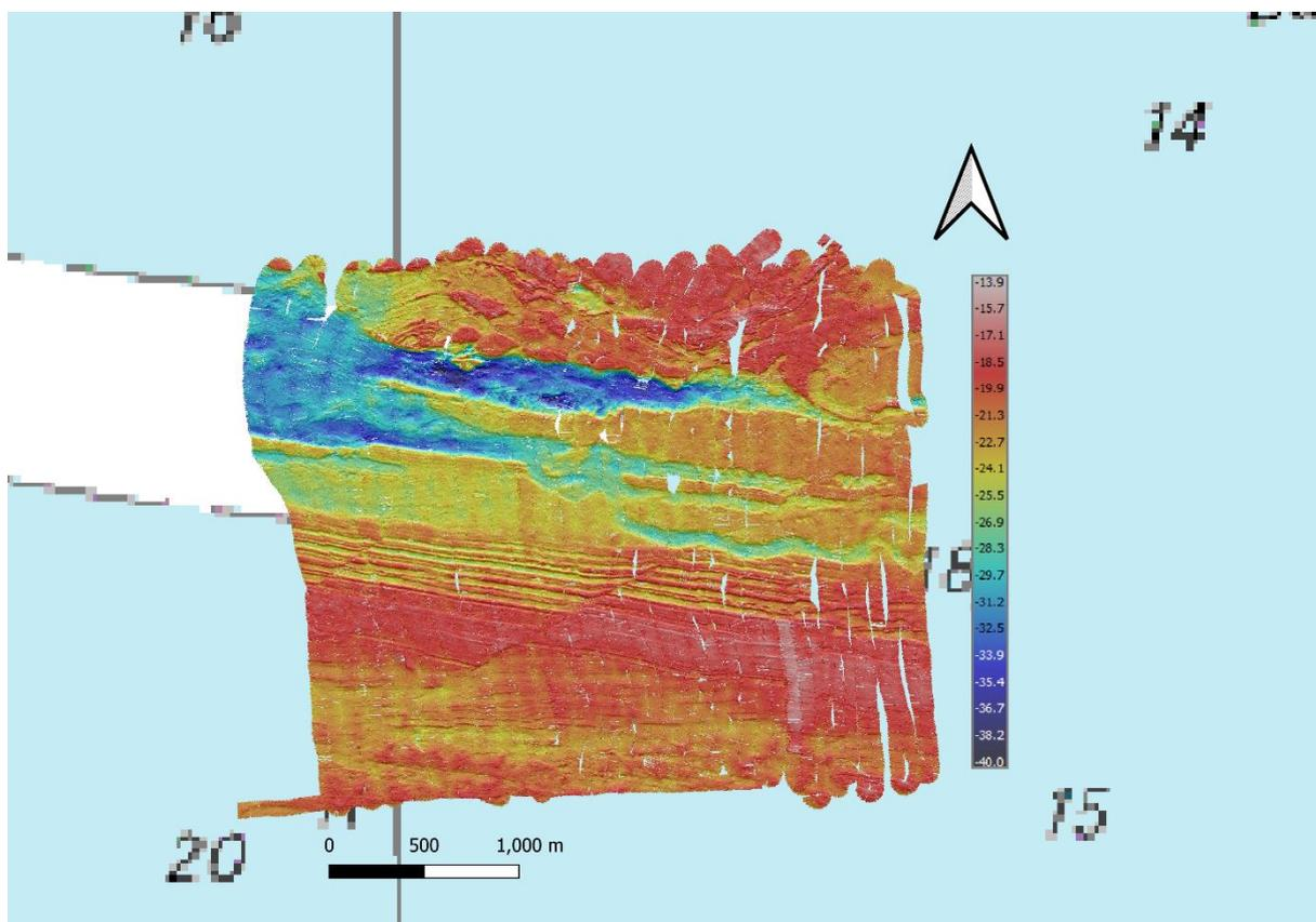
Figure 8. Benthic map of the Frouquie box generated from multibeam sonar surveys. Scale bar shows depth below Chart Datum.
