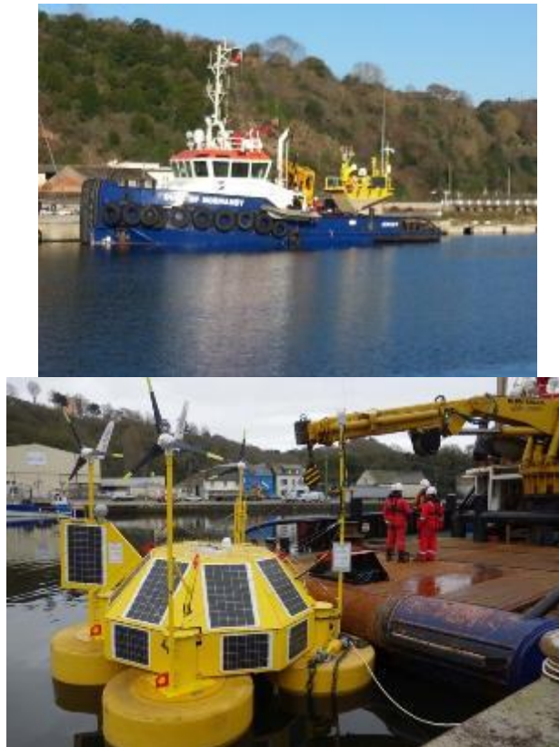
Figure 7-17, Jersey's tug the Duke of Normandy being used to install a floating LiDAR buoy for the St Brieuc offshore wind project.
