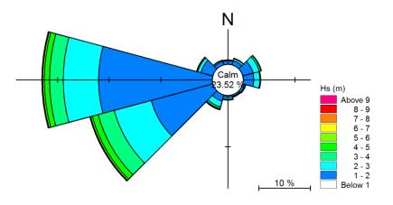
Figure F-2: Wave Rose for UKMO data (significant wave height, Hs)
