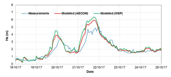
Figure F-13: Calibration of Significant Wave Height (Event 3 – October 2017)
