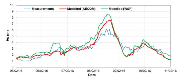
Figure F-7: Calibration of Significant Wave Height (Event 1 - February 2016)
