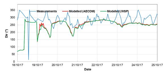
Figure F-15: Calibration of Wave Direction (Event 3 – October 2017)
