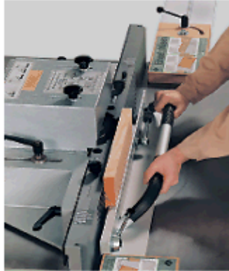
Use of jig for stopped work
