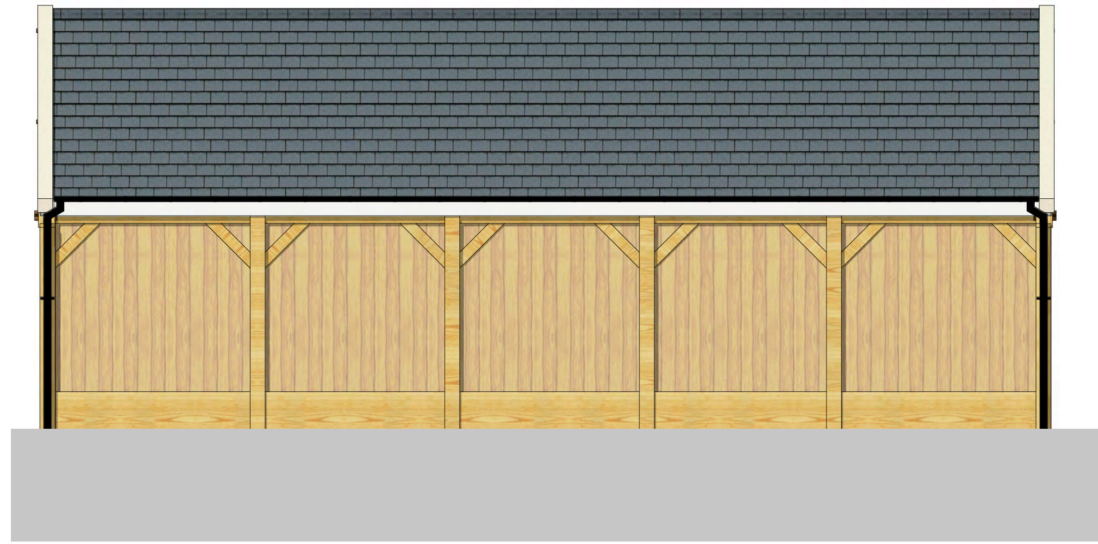
HOUSE 26,27,28 CARPORT SOUTH EAST (REAR) ELEVATION 1:50
