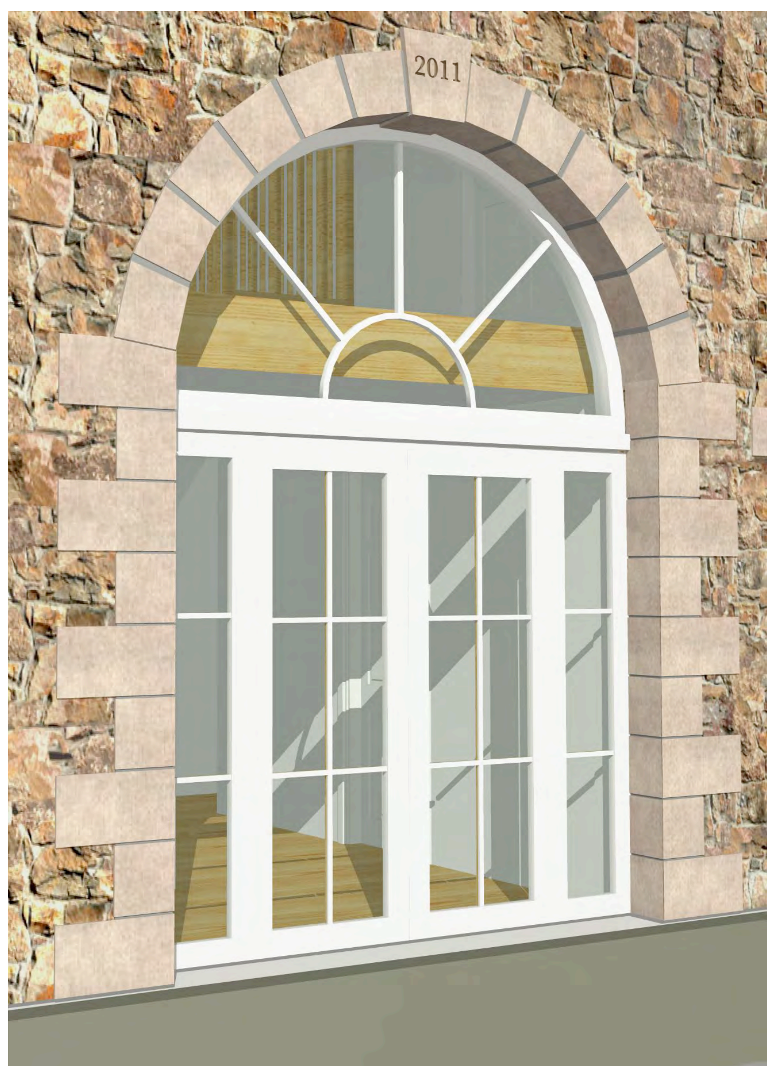
PROPOSED DOORS WITH SIDE LIGHTS AND SEALED WINDOW OVER SEE DWG 1871/P/02
