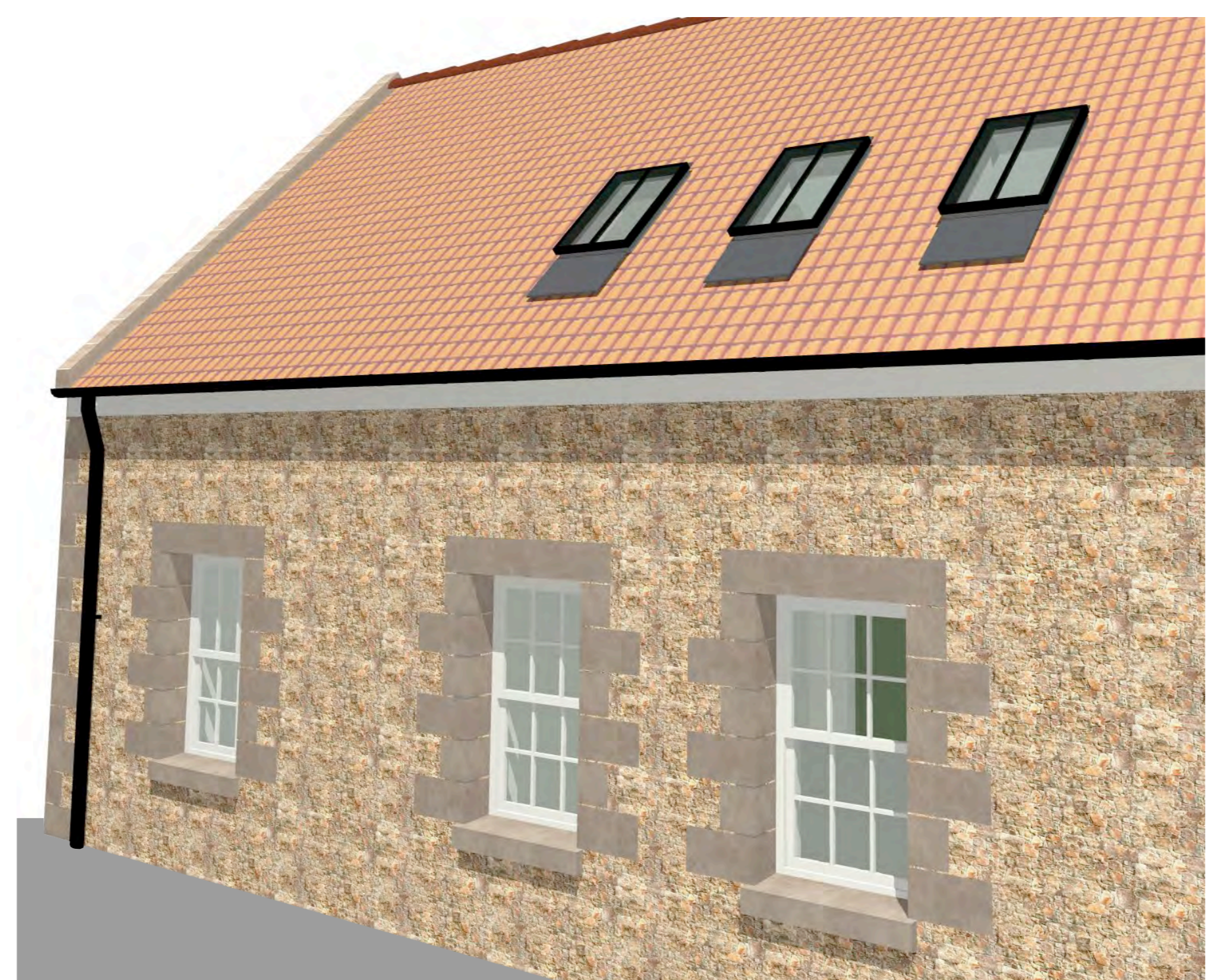
REAR OF GARAGE. GRANITE LINTOLS, QUOINS AND CILLS IN WALLS FINISHED WITH ROUGHLY DRESSED GRANITE. SEE DWG 1871/P/02. CONSERVATION ROOF LIGHTS. SEE DWG 1871/P/02.
