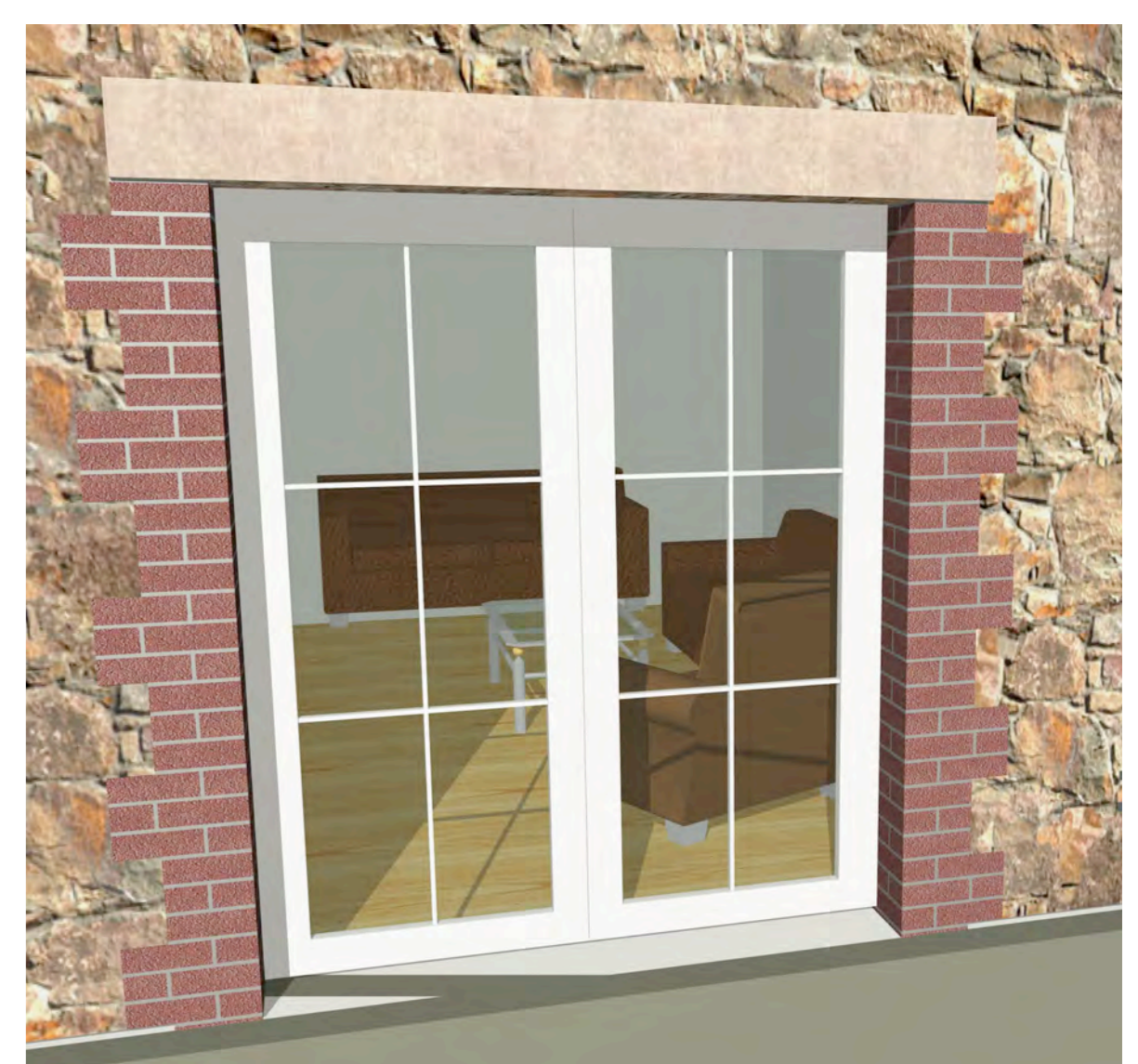
DOUBLE GLAZED REAR FRENCH DOORS WITH BRICK QUIOINS AND GRANITE LINTOL
