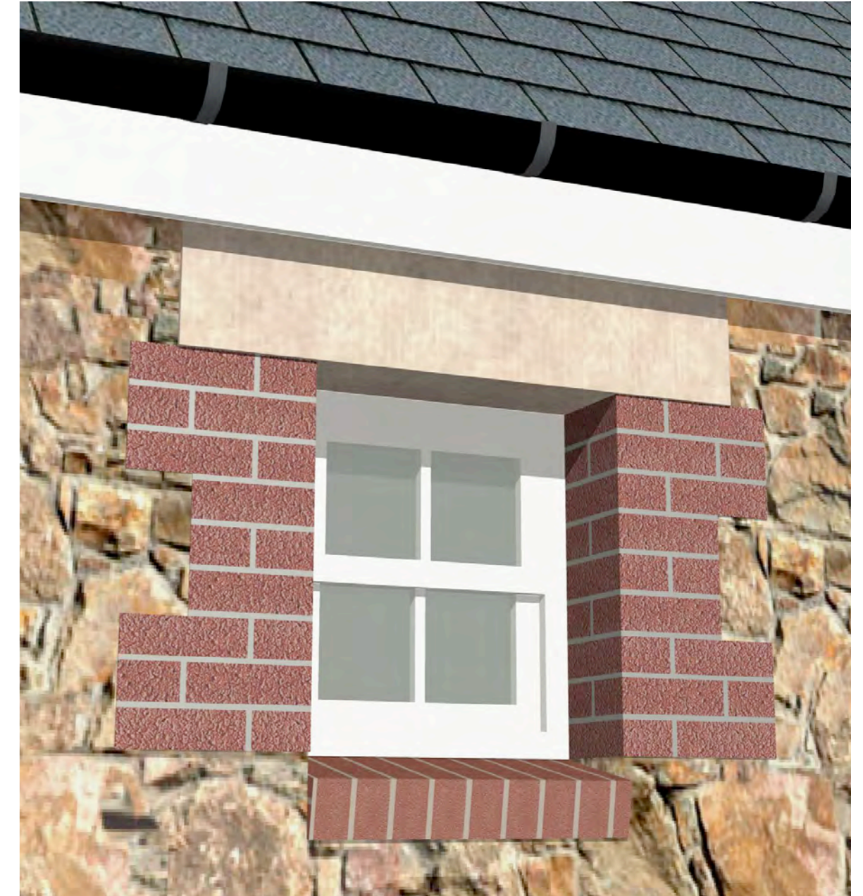
SMALL FIRST FLOOR WINDOW WITH BRICK QUIOINS AND CILL WITH A GRANITE LINTOL
