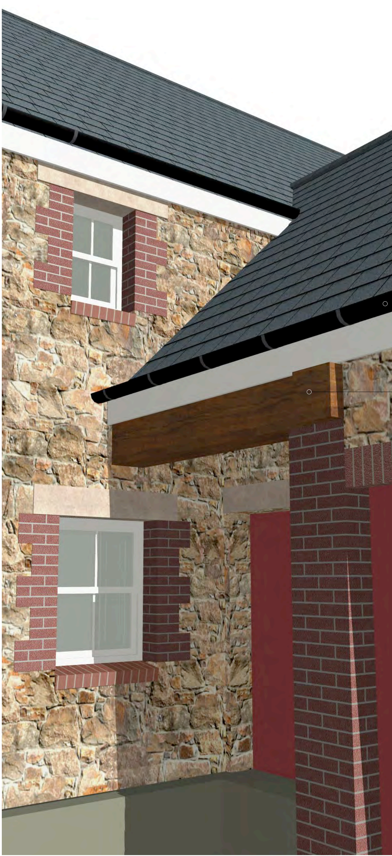
ENTRANCE TO UNIT 3 WITH BRICKWORK CILLS & QUOINS AND BRICK PIERS AND LINTOL TO GARAGES SEE DWG 1871/P/02
