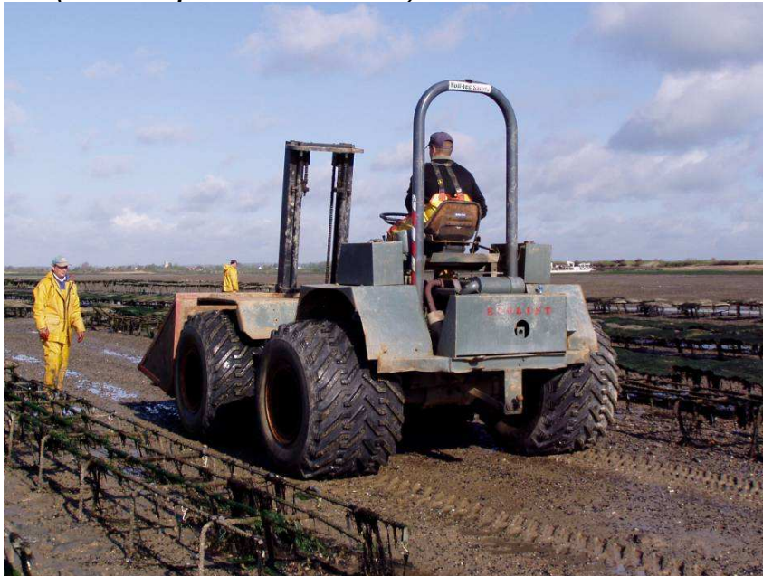
Figure 32. Purpose designed aquaculture tractor with wide tyres for reduced impact on benthos (Source: Aquafish Solutions Ltd.)
