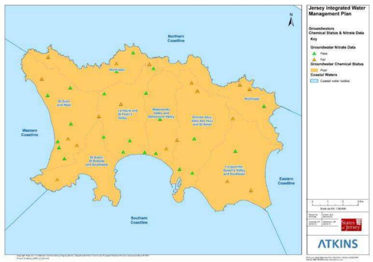
Figure 22: Groundwater Chemical Status and Nitrate Monitoring data
